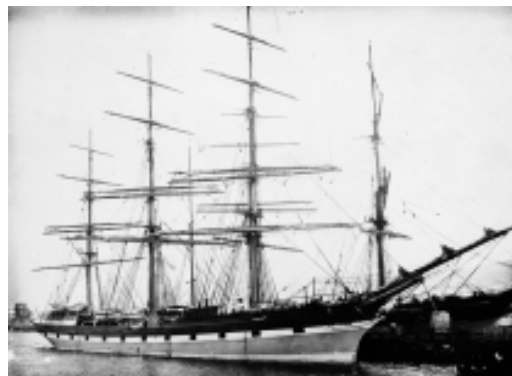
The ship Blenheim , 1077 tons, built in Glasgow in 1877, originally the Wanganui , re-rigged as a barque in 1904
